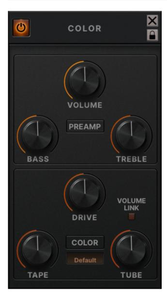
**PREAMP** — Preamp-style filters that precede the Color saturation circuits.
