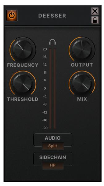
**Frequency**: The target frequency that the module will process.
