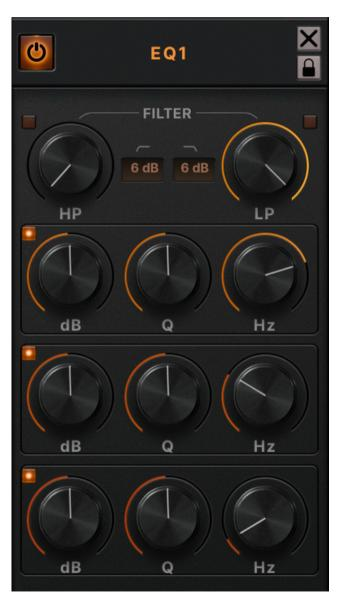
High-pass (HP) & Low-pass (LP) Filters: Toggle the filters on/off state by engaging or disengaging the LED button. The slope of the filter (dB/oct) shows the options as a dropdown menu. These filters are static to their respective filter type.
