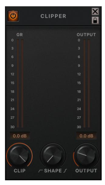
**Clip:** Threshold (dB) of the clipping processor.
