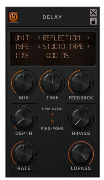
**Low-pass / "LOPASS":** Filters the delayed signal from 500Hz to 22kHz.
